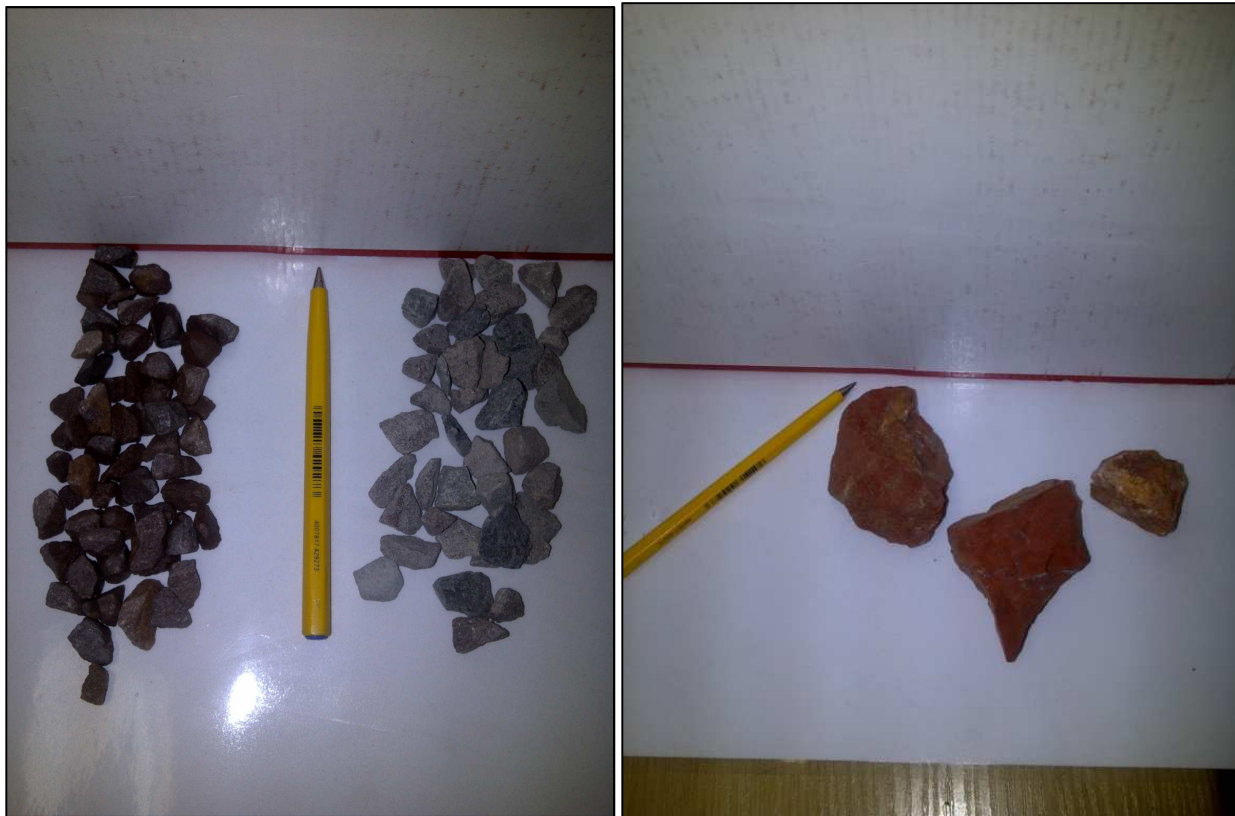
Figure 3: Red Durban Aggregate, Grey Reebok Aggregate and Red Jasper Aggregate (L to R)
