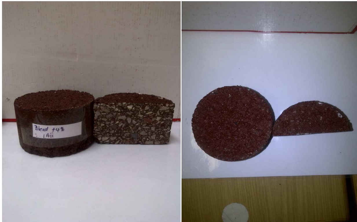
Figure 4: Option 2B(ii) from Table 1 (AC surfacing with red oxide colouring and 50% colour coded aggregate ex Durban)
