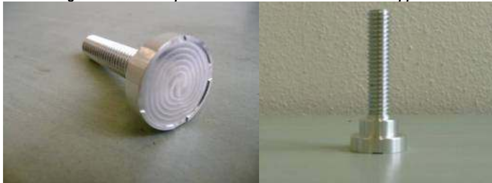
Figure 4 – Modified BBS test pull-out stubs .
