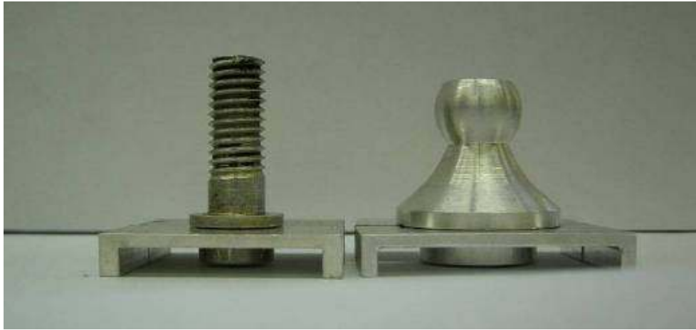
Figure 3 – Modified pull-out stub with aluminum frame supports.
