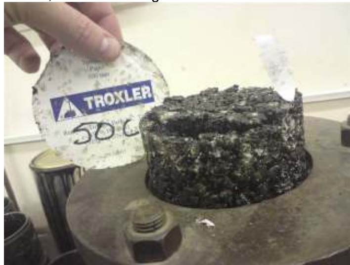
Figure 8: Expansion of shelf life sample after Marshall compaction and conditioning at 30°C.
