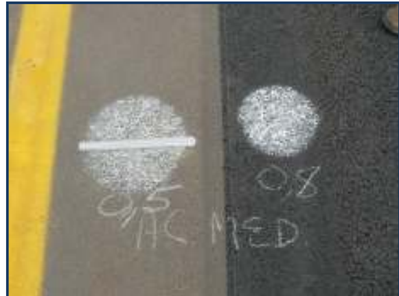
FIGURE 19 : TEXTURE IMPROVEMENT OF AC MEDIUM
