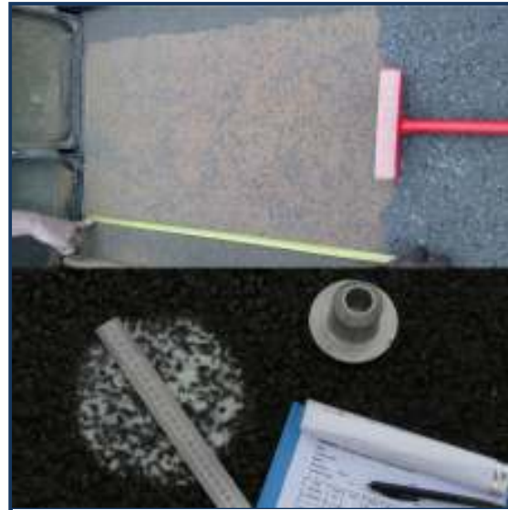
FIGURE 3 : SAND PATCH TEST AND ASC TEST
