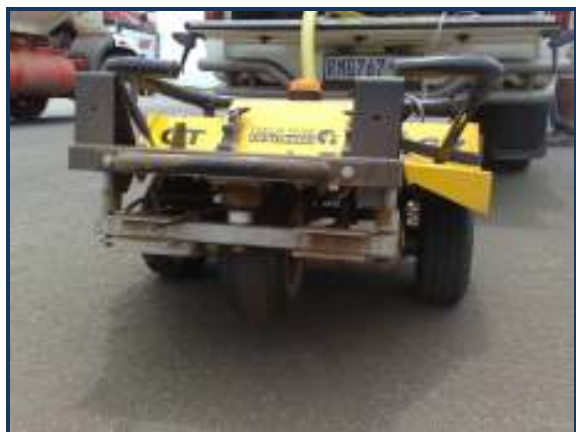
FIGURE 8: VIEW OF GRIP TESTER
