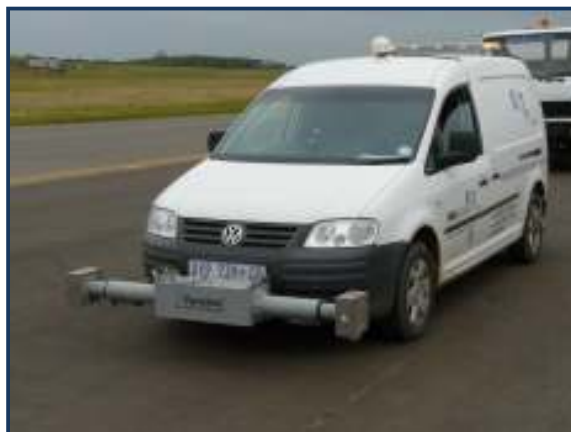
FIGURE 9: VIEW OF DYNATEST ROAD SURFACE PROFILER
