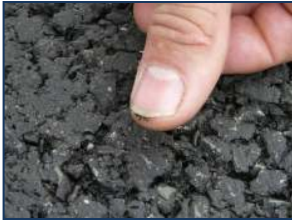
FIGURE 18 : VIEW OF WATER-CUT MACRO-TEXTURE
