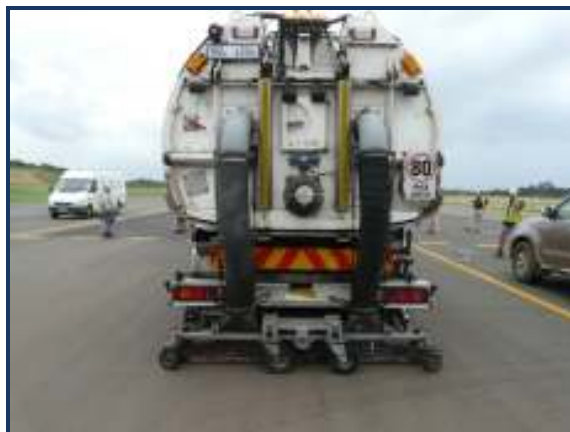
FIGURE 6 : BACKVIEW OF UHP WATER-CUTTER
