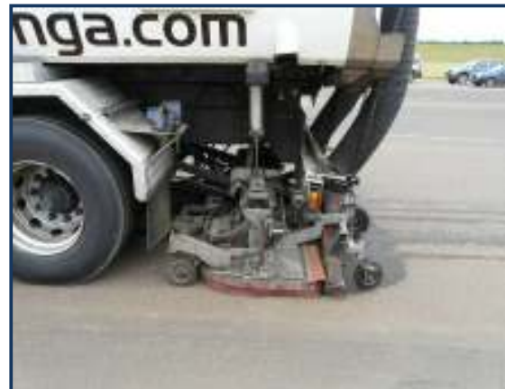
FIGURE 17 : START OF OF LANE1 WATER-CUTTING
