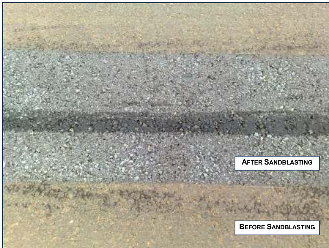
FIGURE 12 : EFFECT OF LIGHT SANDBLASTING ON THE SURFACE TEXTURE OF THE SMA WEARING COURSE
