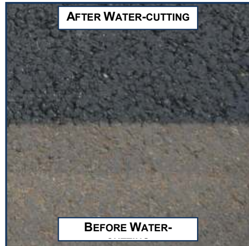
FIGURE 5 : EFFECT OF WATER-CUTTING ON TEXTURE
